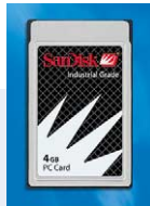
PCMCIA PC Card Type II height 5,0 mm
